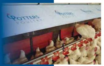
The standard single tier system boasts a variable speed egg belt for complete control of egg collection.
