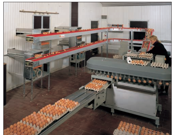
The eggs are transported via a rod curve conveyor to the egg packer
