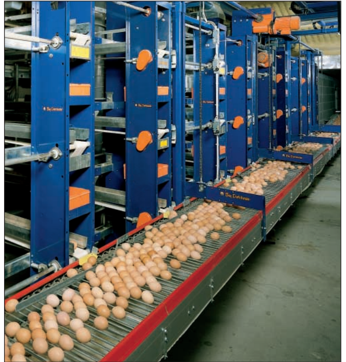
Lift system – eggs are collected by tier
