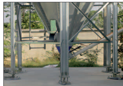
Silo scale with electronic load cells
